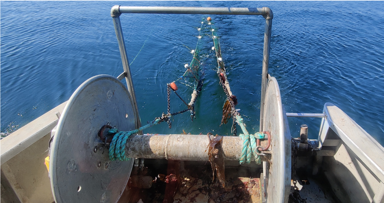
Figure 3. Small-scale Danish seine net being set during gear trials in the Storebælt (Great Belt). © Thomas Noack.
