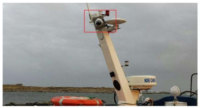
Figure 2. CCTV cameras installed on a small inshore commercial fishing vessel.
