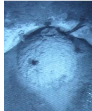
Figure 30: Two sea mines, originally laid on the same day and found in the middle of the Baltic Sea within a distance of approximately 1400 meter of each other, exemplify the differences in state of corrosion of encountered munitions (Wichert 2012).
