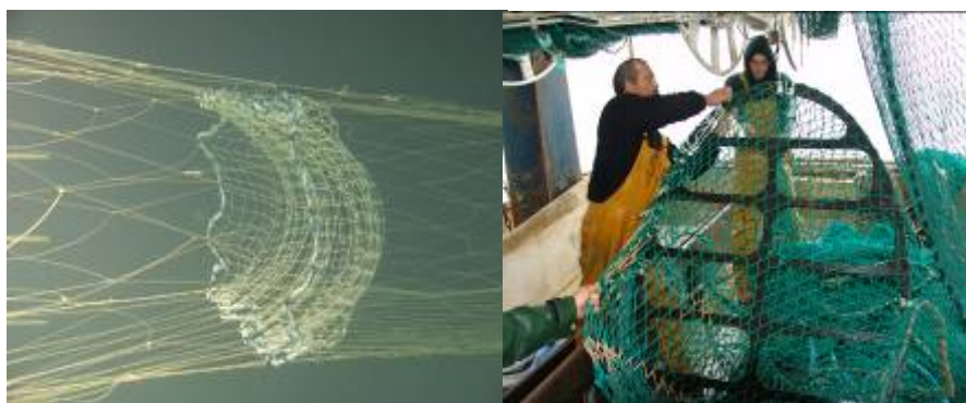
Figure 5. A vertical net barrier and a flexible semi-oval grid as tested by IFREMER
