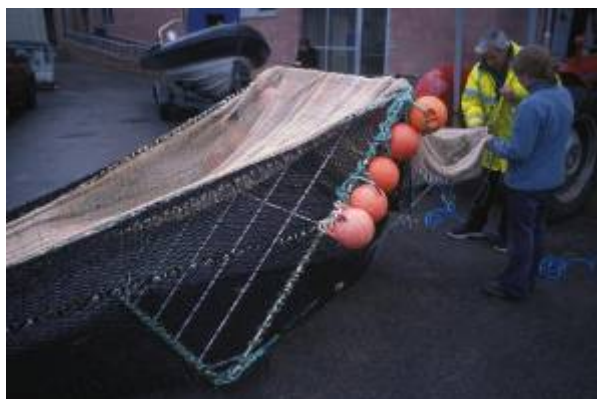
Figure 4. Steel exclusion grid with 1.7m escape hatch and 22mm netting cover
