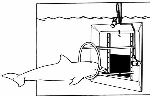
**Figure 55: Tests on dolphin behaviour under deterrent signals in Brughes, Belgium – experimental set-up**
