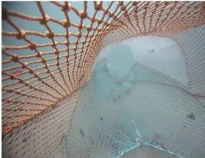
**Figure 20: Underwater footage of Inclined Separator Panel**
