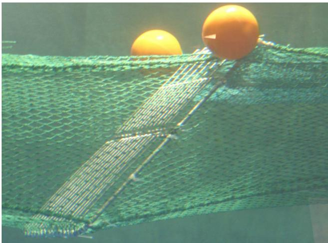
**Figure 3: Grid used in Danish Nephrops fishery – model**
