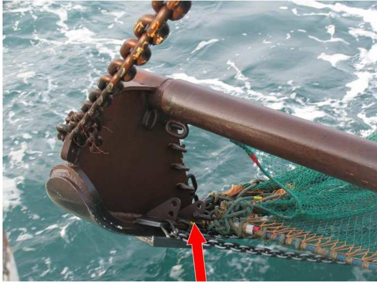
**Figure 21: Lowered headline in Nephrops Beam Trawl**
