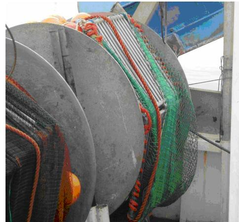
**Figure 2: Grid used in Swedish Nephrops fishery – on the netdrum**
