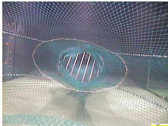
**Figure 49: Grid configurations tested in the flume tank of Boulogne, France by IFREMER - flexible version**
