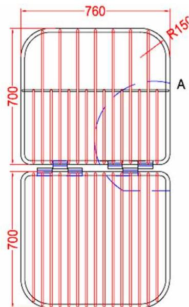
**Figure 4: Grid used in Danish Nephrops fishery – dimensions**
