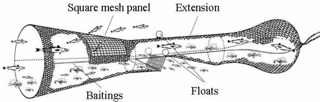
**Figure 5: Principle of panel and grid in the Bay of Biscay**
