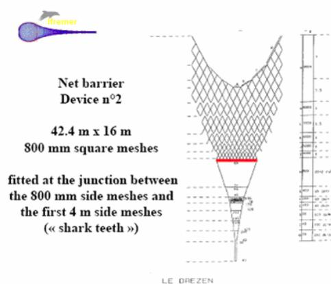
**Figure 45: Design of net barrier by IFREMER – LE DREZEN**
