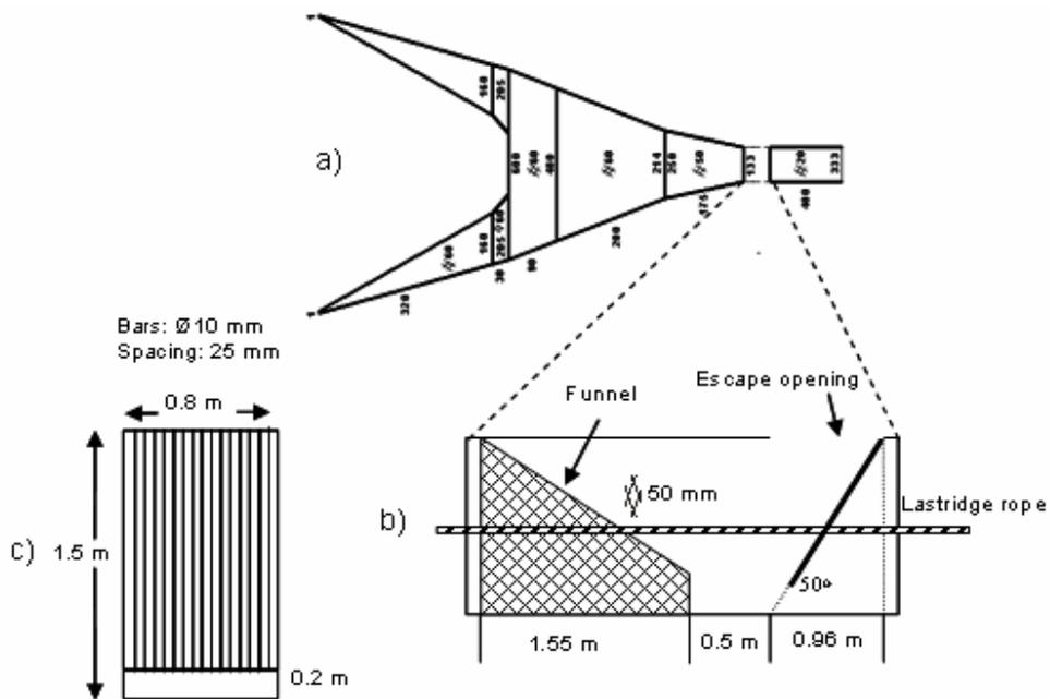
Figure 9: Grid sorting system (GCRUST1) tested in Portuguese Nephrops fishery
