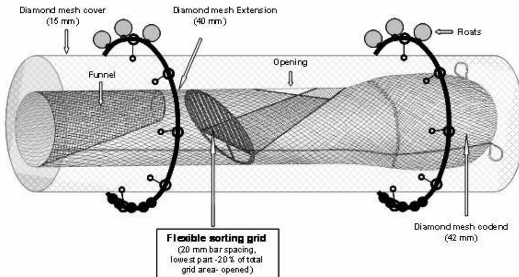
Figure 14: Sorting grid with guiding funnel used in the Catalan Sea
