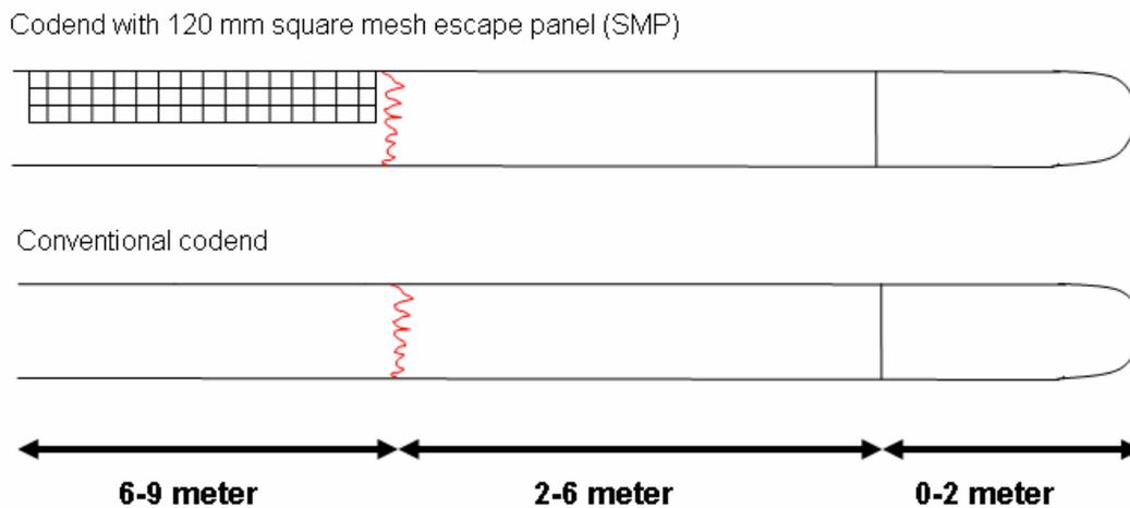
Figure 15: SMP and conventional codend used in Denmark
