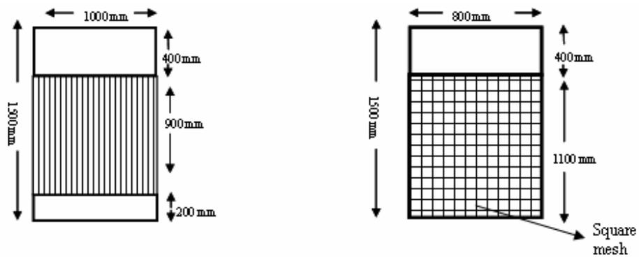
Figure 10: Grids (GCRUST2 and GCRUST3) tested in Portuguese Nephrops fishery - alternative designs
