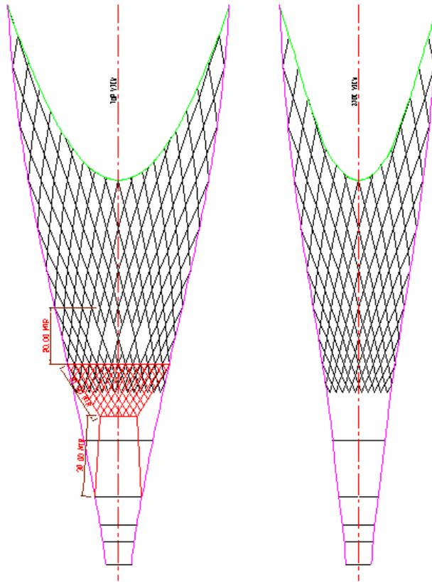
**Figure 43: Tunnel barrier designed by IMARES and MARITIEM, tested on FRV “Walther Herwig - III” in 2006.**
