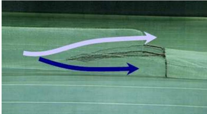
**Figure 19: Inclined Separator Panel – model showing working principle. Light blue arrow is non-target species, dark blue is target species**
