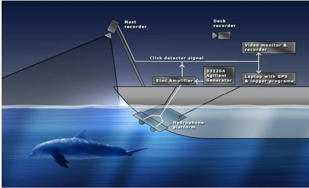
**Figure 52: Tests on dolphin behaviour under deterrent signals by DIFRES in Alboran Sea – experimental set-up 1**
