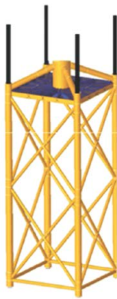
Figure 26: Concept of a quadjack foundation with Pile-in-Pipe Piling for the application with an offshore wind turbine (source: OVERDICK GmbH & Co. KG, Hamburg, modified)
