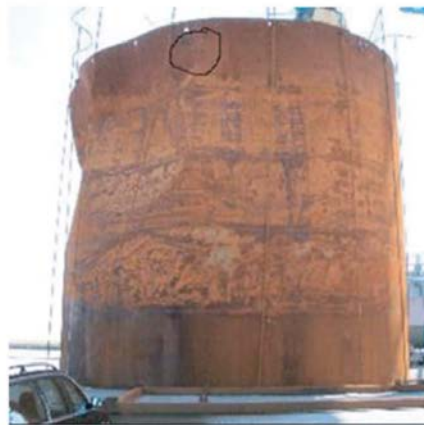
Figure 65: Deformed bucket foundation of an Enercon E 112 wind turbine near Hooksiel (source: IBSEN & NIELSEN 2007)
