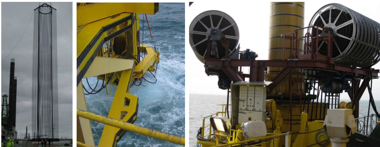
Figure 12: Little bubble curtain of vertical hoses (SBC of MENCK/BARD ). Concept tested at OFT 1 (left and middle, see text) and improved concept for OFT 2 (right) (source: STEINHAGEN 2012)
