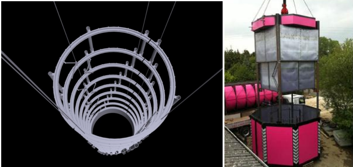
Figure 11: Layered and confined bubble curtain by Weyres Offshore . Principle of the layered arrangement of the pipes (left) (source: http://www.weyres-offshore.de/ ) and telescopic extended system (right) (source: WILKE et al. 2012, photo: B. WEYRES)
