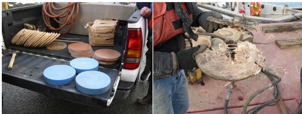
Figure 34: Piling cushions tested in the experiments by the Washington State Department of Transportation before being used (left), and fractured and compressed plywood piling cushion after being used (right) (source: LAUGHLIN 2006)
