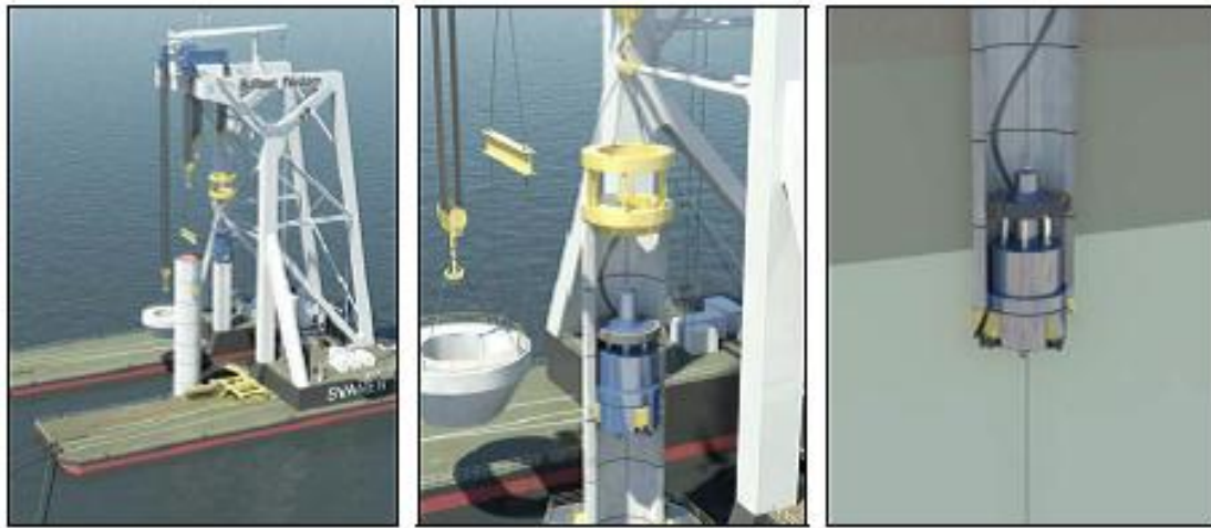
Figure 43: Drilled concrete monopile concept of Ballast Nedam : positioning (left), drill head before installation within the monopile (middle), drilling operation and penetration of the monopile (right) (source: VAN DE BRUG 2011)
