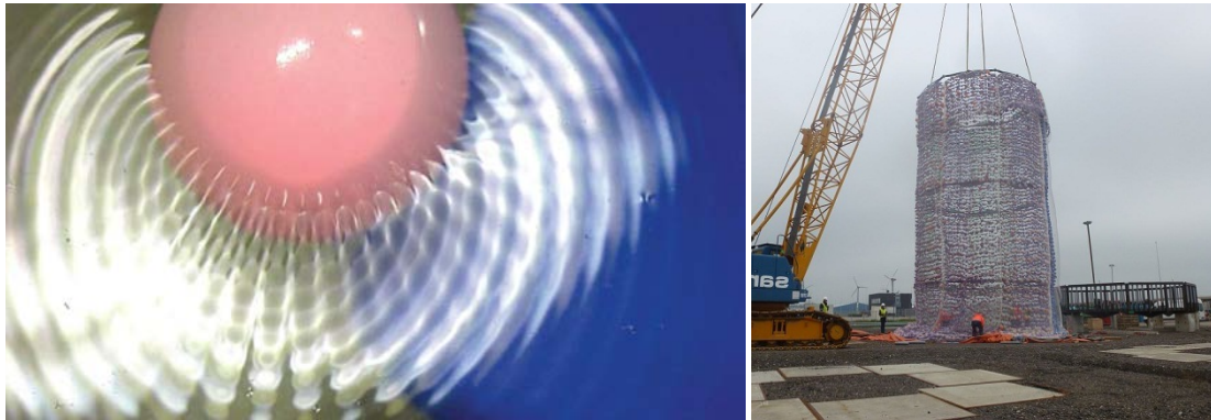
Figure 30: Scattering and absorption tests with HSD balloons in a wave flume (left) and preparations for practical application of an HSD net ( \varnothing 9m, height 28 m, weight of the complete system 17 t) at the OWF London Array (right) (sources: ELMER et al. 2011, 2012)
