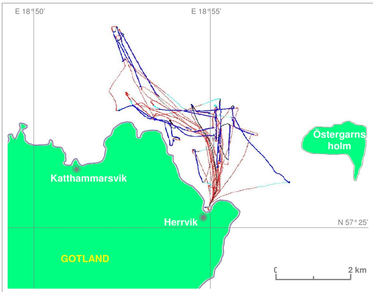
Plate 4. Sensor data shown in map format with each fishing activity shown in a different colour as defined by the vessel's velocity and other data. Solid dark blue shows net hauling, dotted red lines are transports between fishing operations and light blue is the time after hauling when the system is still recording. This map shows a few trips with Boat 2 in early June.
