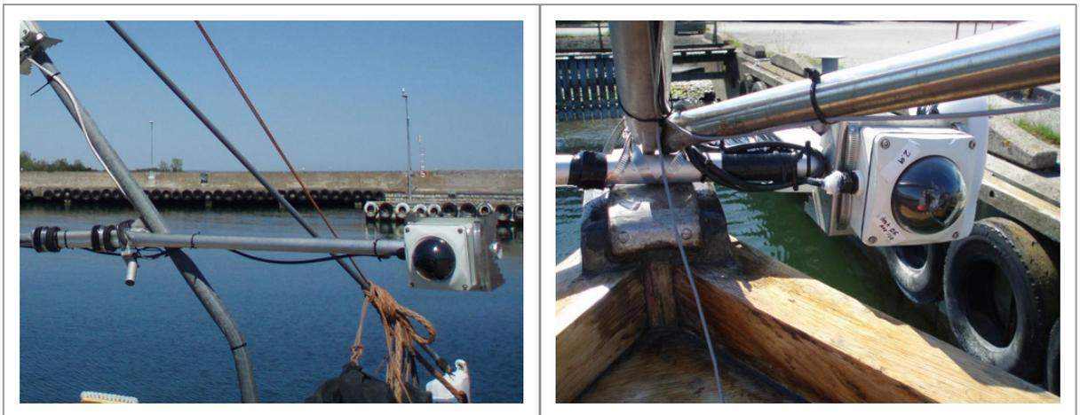
Plate 2. Temporary constructions for mounting 'outrigger' cameras in order to document any by-catches which might fall out of the nets before arriving at the hauler; on 'Boat 2' (left) and 'Boat 1' (right).
